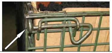
This basket is not properly latched. The end of the latch is not through the tongue. Make sure that the tongue is properly engaged in the side of the wiretainer before latching.
