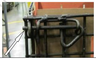
The latch in this photo is properly engaged. The latch passes through the tongue. The latch handle must be pointing down.
